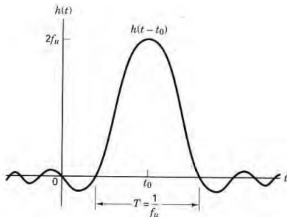
**Figure 1.12** Impulse response of the ideal low-pass filter.
