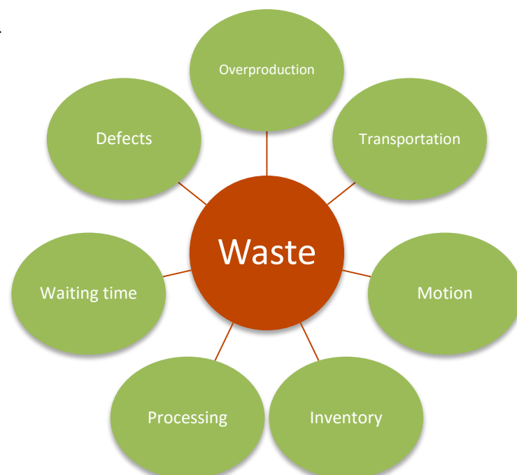
Fig. 1 The seven categories of waste. Source: Adapted from Asefeso [6].
