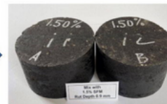
Making HMA samples containing face masks
