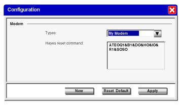
The selected configuration corresponds to the one read in the controller: the Hayes initialization command, then read, is displayed in Hayes standard format.
